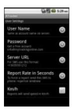
The User Name and Password are supplied by the map server administrator. The field under the password is the Server URL of the map server. NOTE: to send reports using SMS, enter the phone number of the GSM modem that will be receiving the reports. Be sure to prefix the phone number with a "+". For example: +13035551212.
